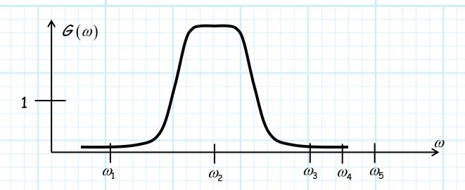
Therefore, the gain in the pass-band is large  $(G(\omega) \gg 1)$ , while outside the pass-band the gain is small  $(G(\omega) \ll 1)$ .
