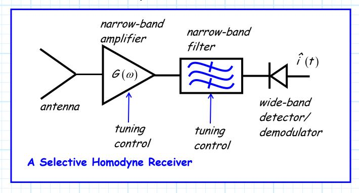
Therefore, if we tune **both** the amplifier and filter to frequency  $\omega_4$ , we might get:
