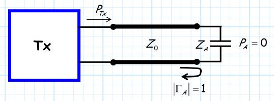
Thus, it is imperative that the impedance of an antenna have a **real** component if we wish for it to **absorb** energy, with maximum power transfer occurring when  $Z_A = Z_0$ .
