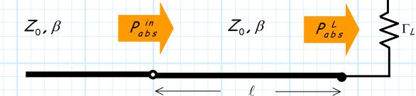
Recall, however, that a lossless transmission line can absorb **no** power! By adding a length of transmission line to load  $\Gamma_L$ , we have added only **reactance**. Therefore, the power absorbed by load  $\Gamma_{in}$  is **equal** to the power absorbed by  $\Gamma_L$ :
