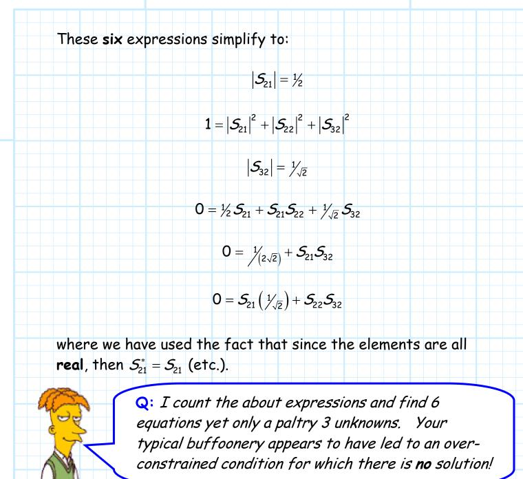
A: Actually, we have six real equations and six real unknowns, since scattering element has a magnitude and phase. In this case we know the values are **real**, and thus the phase is either 0° or 180° (i.e.,  $e^{j0} = 1$  or  $e^{j\pi} = -1$ ); however, we do not know which one!
