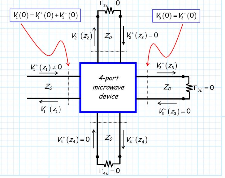
Typically, it is **much** more difficult to determine/measure the scattering parameters of the form  $S_{nn}$ , as opposed to scattering parameters of the form  $S_{mn}$  (where  $m \neq n$ ) where there is **only** an **exiting** wave from port m!
