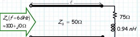
6) Determine the proper value for line length  $\ell$ . Now replace the 100  $\Omega$  resistor with this 100  $\Omega$  "load" shown above, and reanalyze (with ADS) each matching transformer design.
