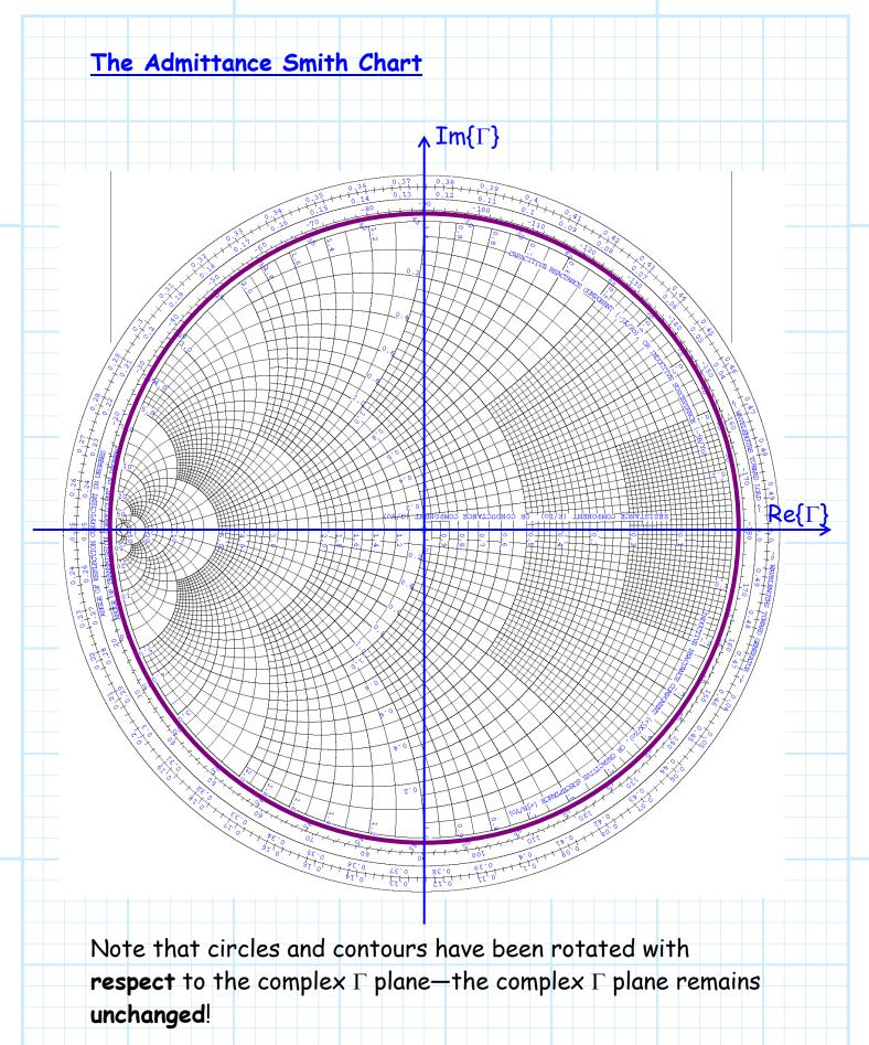
This result should **not** surprise us. Recall the case where a transmission line of length  $\ell = \lambda/4$  is terminated with a load of impedance  $z'_{\ell}$  (or equivalently, admittance  $y'_{\ell}$ ). The input impedance (admittance) for this case is:
