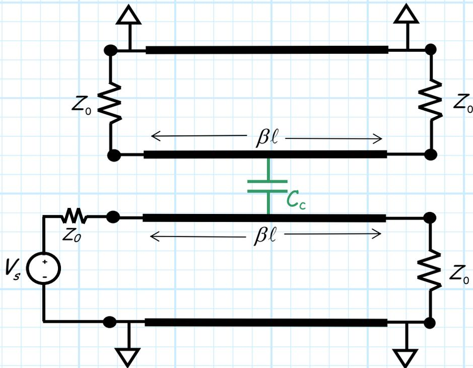
Typically, a coupled-line coupler schematic is drawn **without** explicitly showing the **ground conductors** (i.e., without the ground plane):
