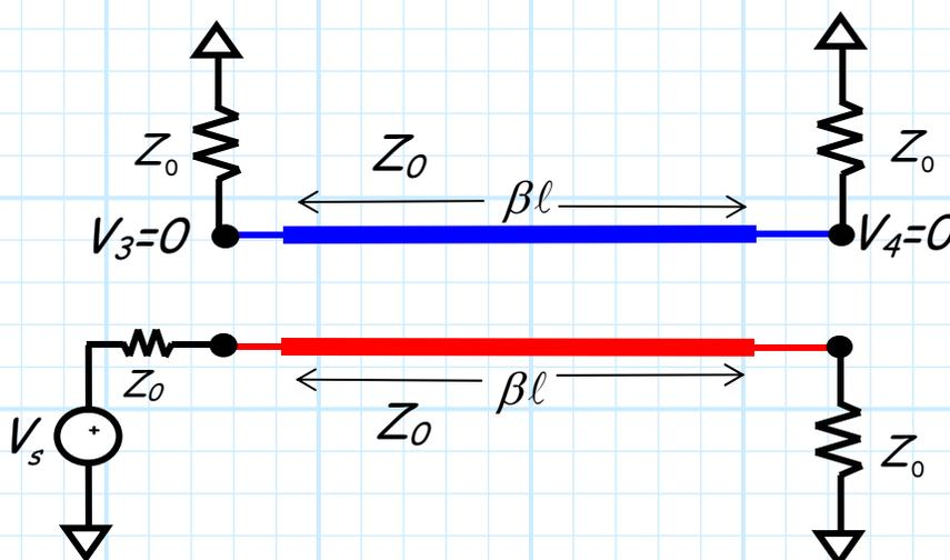
This makes sense! After all, if no coupling occurs, then the characteristic impedance of each line is **unaltered** by the presence of the other—their characteristic impedance is  $Z_0$  **regardless** of “mode”.
