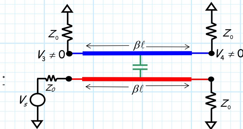
Now, our **first step** in performing the odd/even mode analysis will be to determine scattering parameter  $S_{11}$ . To accomplish this, we will need to determine voltage  $V_1$ :
