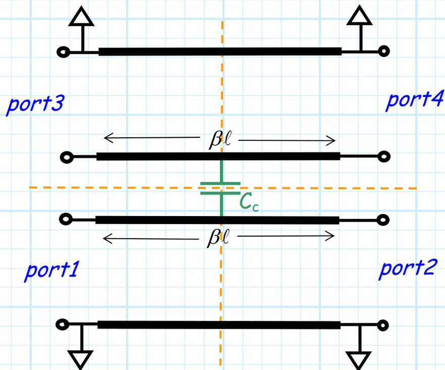
As a result, we know that the **scattering matrix** of this four-port device has just **4 independent** elements:
