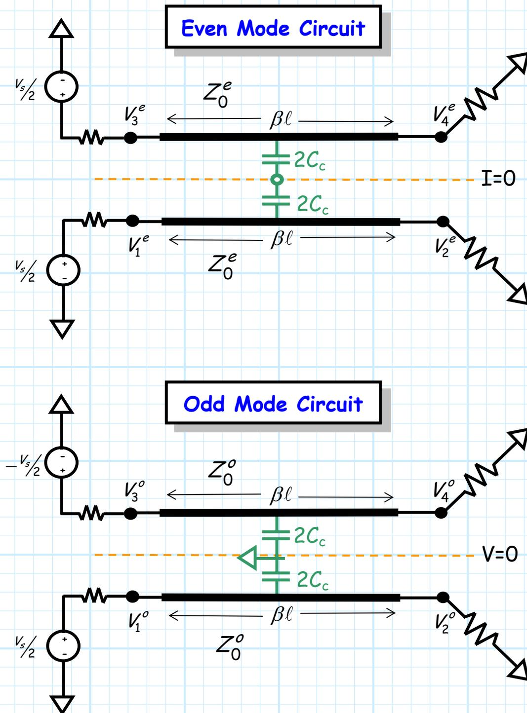
Note that the **capacitive coupling** associated with these modes are different, resulting in a **different** characteristic impedance of the lines for the two cases (i.e.,  $Z_0^e, Z_0^o$ ).
