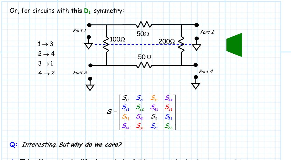
A: This will greatly simplify the analysis of this symmetric circuit, as we need to determine only six matrix elements!
