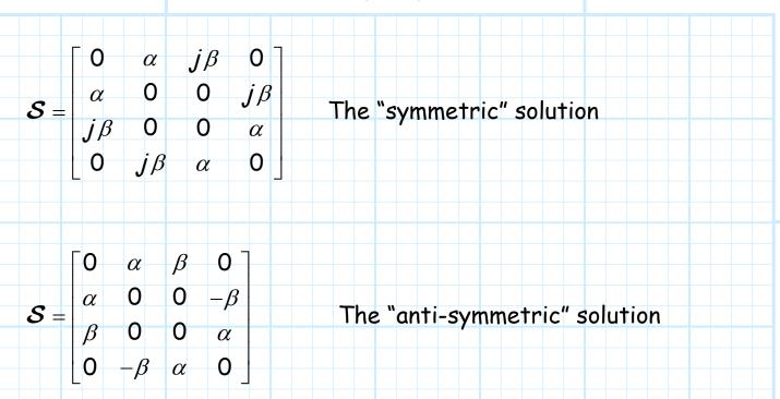
**Compare** these to the matrix forms above. The "symmetric solution" has the same form as the scattering matrix of a circuit with  $D_2$  symmetry!
