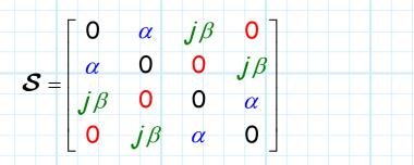
**Q:** Does this mean that a matched, lossless, reciprocal fourport device with the "symmetric" scattering matrix **must** exhibit **D**<sub>2</sub> symmetry?
