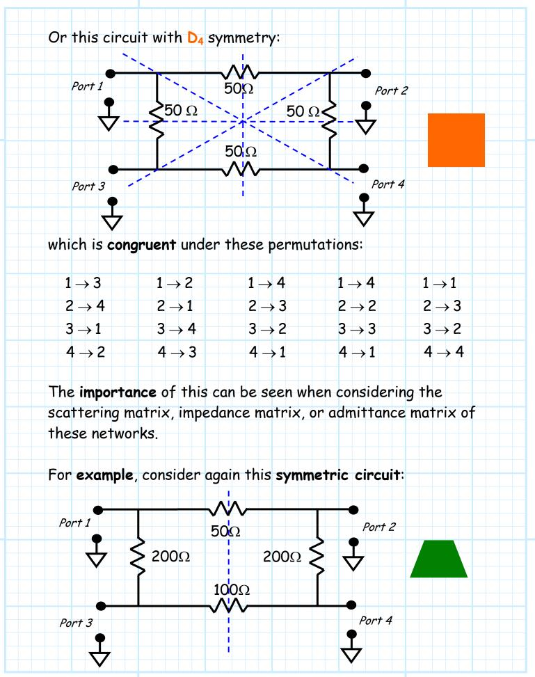
This four-port network has a single plane of **reflection** symmetry (i.e.,  $D_1$  symmetry), and thus is congruent under the permutation:
