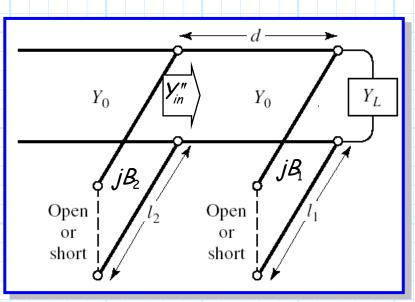
In this design, d is a **fixed** length (typically,  $d = \lambda/8$ ), whereas lengths  $\ell_1$  and  $\ell_2$  are **design parameters**.
