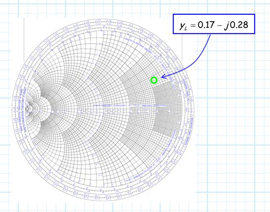
Thus, use the **admittance** mapping at that point to determine the admittance value of  $\Gamma_{L}$ .
