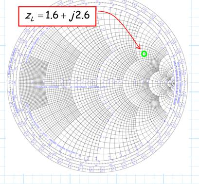
Then, we can rotate the **entire** Smith Chart 180°--while keeping the point  $\Gamma$ , location on the complex  $\Gamma$  plane **fixed**.
