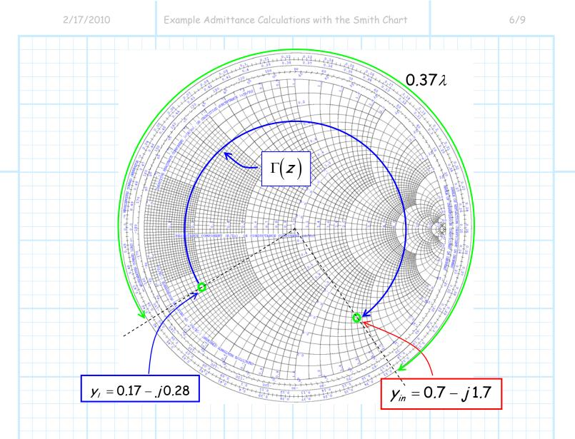
**Transforming** the load admittance to the beginning of the transmission line, we have determined that  $y'_{in} = 0.7 - j1.7$ .
