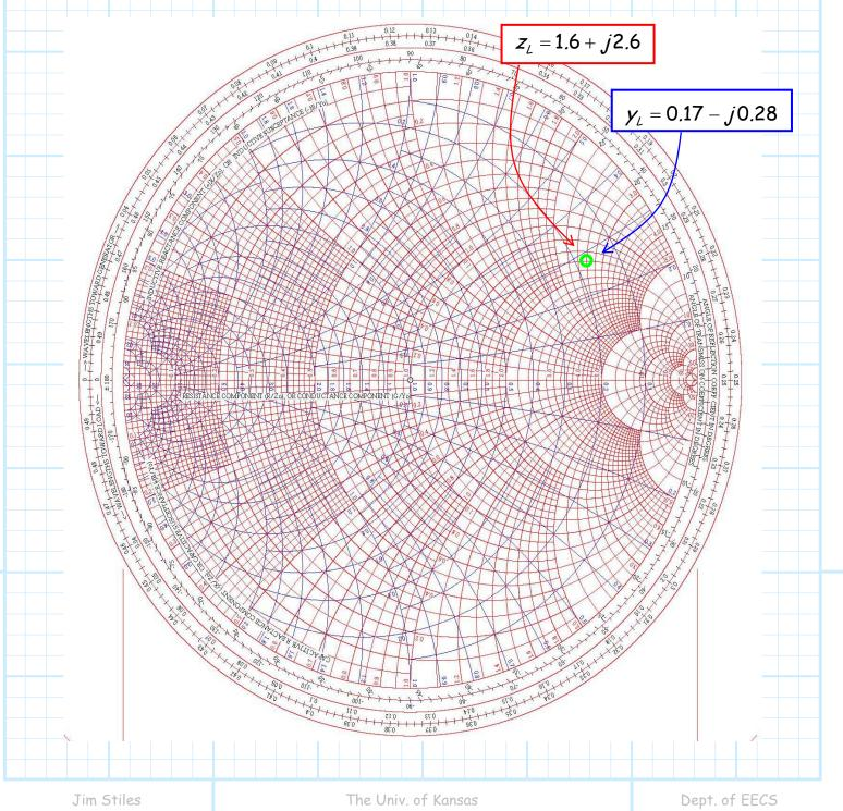
The Smith Chart above shows both the impedance mapping (red) and admittance mapping (blue). Thus, we can locate the impedance  $z_{L} = 1.6 + j2.6$  on the impedance (red) mapping, and then determine the value of that same  $\Gamma_{L}$  point using the admittance (blue) mapping.
