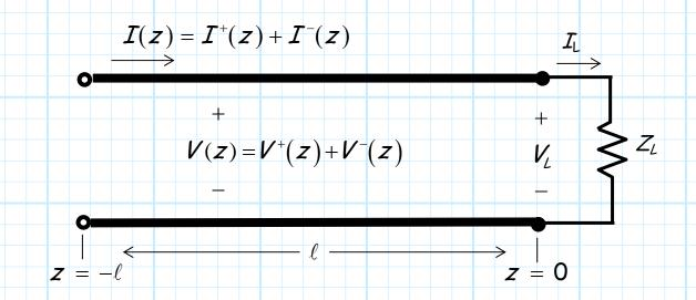
The result is that electromagnetic energy flows along the transmission line at a given rate (i.e., power).
