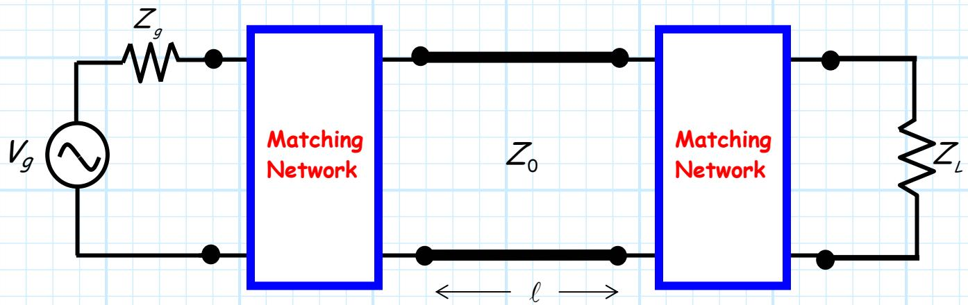
The first network matches the **source** to the transmission line—in other words, it transforms the **output impedance** of the equivalent source to a value numerically equal to **characteristic impedance**  $Z_0$ :
