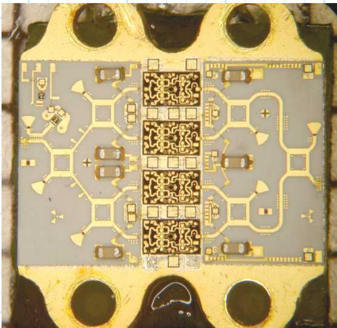
technology. Microstrip circuits are constructed on ceramic or crystalline substrates, typically with low loss and high dielectric constant. Components such as chip resistors and conductors can be attached, as well as individual integrated circuits.
