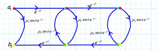
Now, we **could** reduce this signal flow graph even further—**or** we could truncate a **propagation series** by considering only the **direct paths!**
