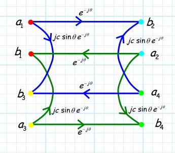
Now, say we cascade three coupled line pairs, to form a three section coupled line coupler. The signal flow graph would thus be:
