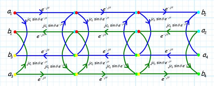
Note that this signal flow graph decouples into two separate and graphs (i.e., the blue graph and the green graph).
