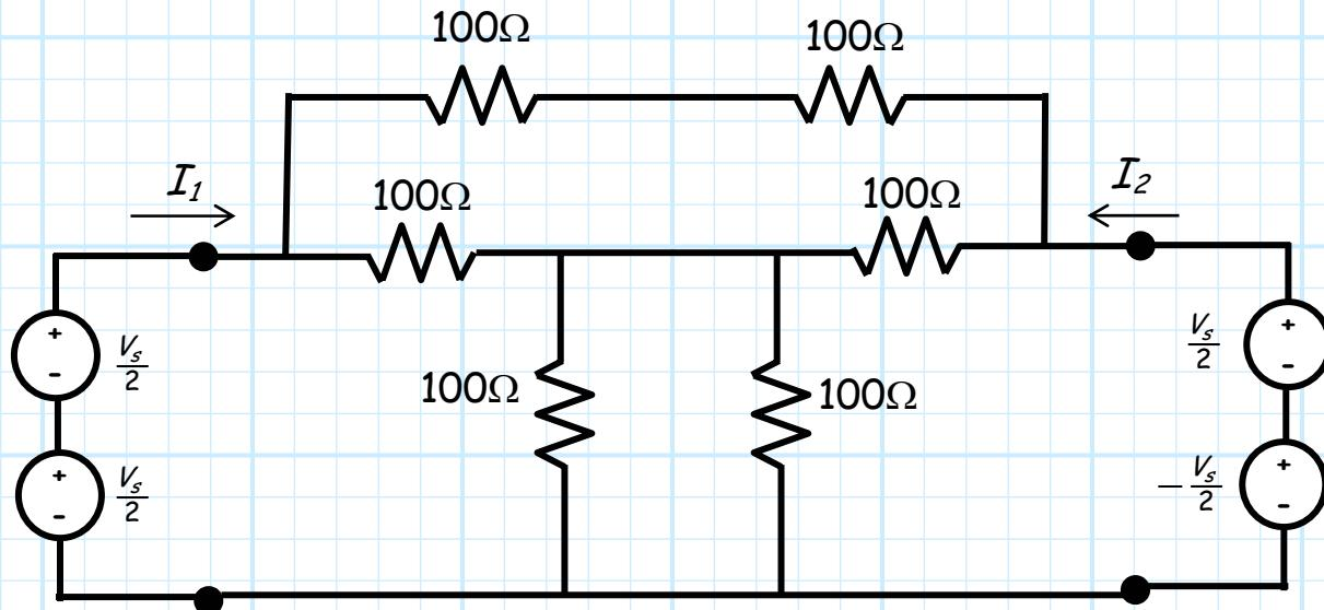
Now, the above circuit (due to the sources) is obviously **asymmetric**—no virtual ground, nor virtual short is present. But, let's say we turn off (i.e., set to  $V=0$ ) the bottom source on each side of the circuit:
