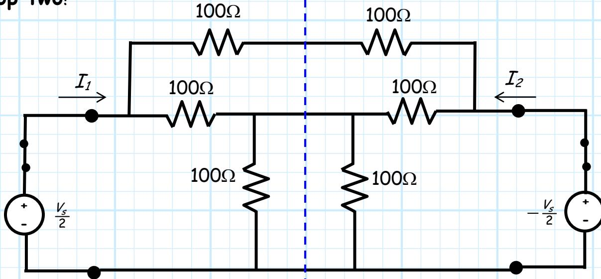
We now have a circuit with **odd symmetry**—the symmetry plane is a **virtual short**!
