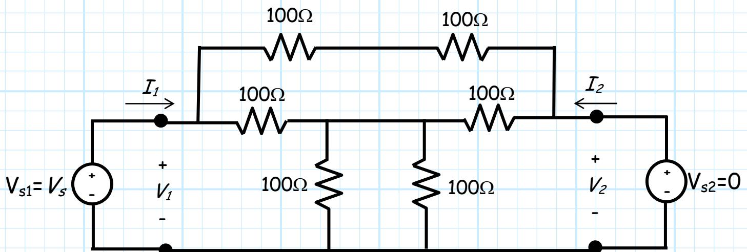
Here's the really **neat** part. We find that the source on port 1 can be modeled as **two equal** voltage sources in series, whereas the source at port 2 can be modeled as **two equal but opposite** sources in series.
