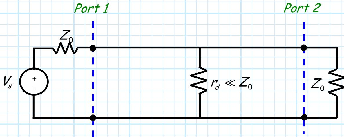
Note that  $|S_{11}| \approx 1$  and  $|S_{21}| \approx 0$  for this case, so that the switch has clearly **disconnected** the source from the load. Likewise, the input impedance of this switch has a very small magnitude—effectively a **short circuit**.
