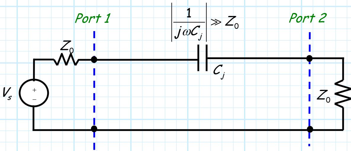
Note that  $|S_{11}| \approx 1$  and  $|S_{21}| \approx 0$  for this case, so that the switch has clearly **disconnected** the source from the load. Likewise, the input impedance of this switch has a very large magnitude—effectively an **open circuit**.
