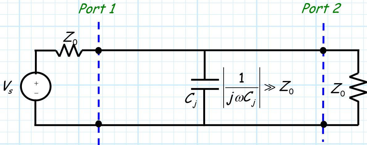
Note that  $|S_{11}| \approx 0$  and  $|S_{21}| \approx 1$  for this case, so that the switch has clearly connected the source to the load.
