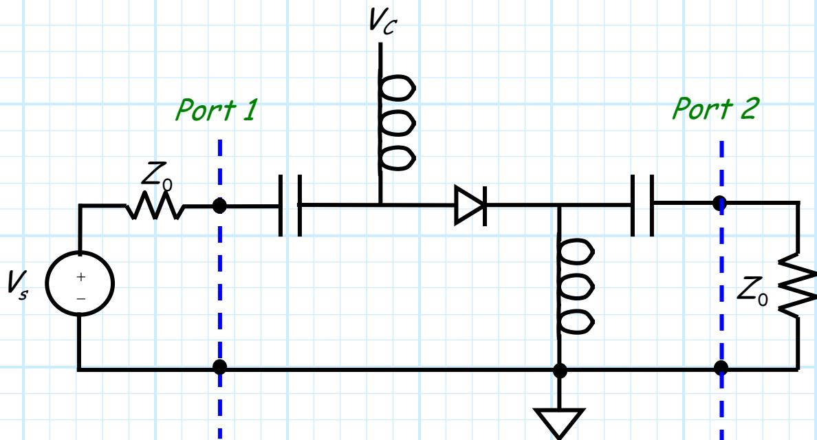
Here the inductors are **microwave chokes** and the capacitors are **DC blocking capacitors**.
