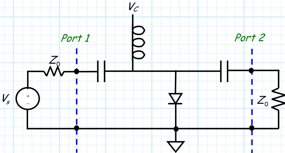
where the inductors are **microwave chokes** and the capacitors are **DC blocking capacitors**.
