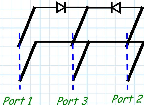
While an **absorptive switch** could be constructed as (where again the DC bias elements have been ignored):
