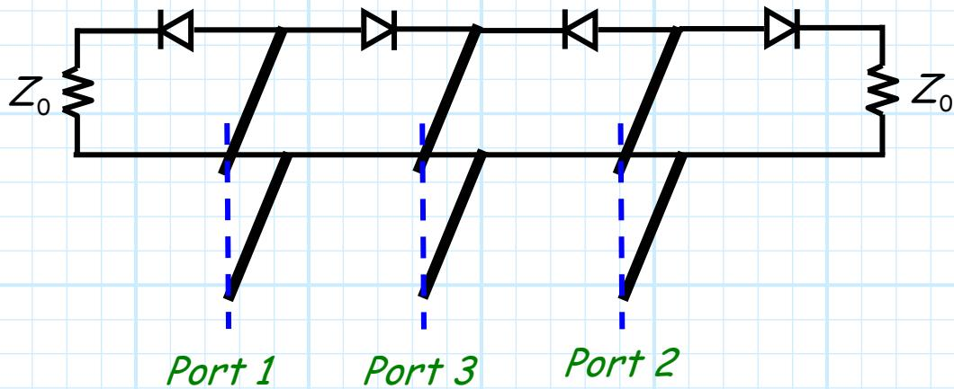
In this case, the port (1 or 2) disconnected from port 3 is connected to a **matched load**.
