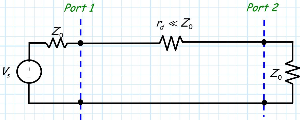
Note that  $|S_{11}| \approx 0$  and  $|S_{21}| \approx 1$  for this case, so that the switch has clearly **connected** the source to the load.
