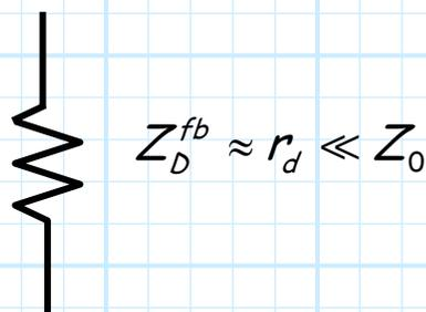
For reverse bias, where  $r_d$  is **very large**, we find that diode impedance  $Z_D$  is approximately equal to that of the junction capacitance  $C_j$ :
