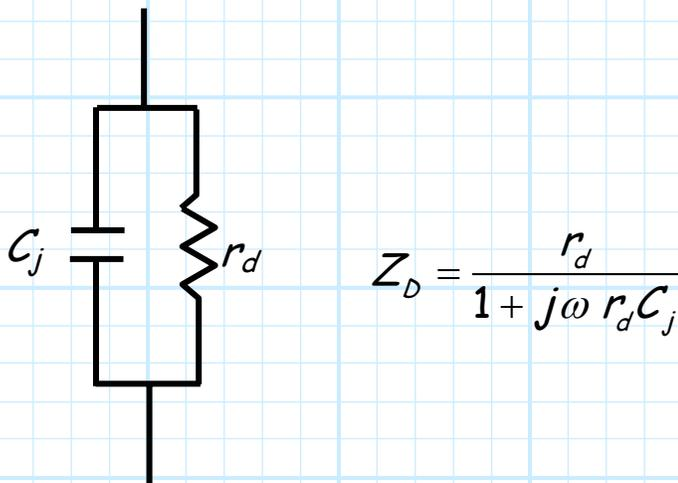
For **forward** bias, where  $r_d$  is **very small**, we find that diode impedance  $Z_D$  is approximately equal to this **small series resistance** ( $Z_D \approx r_d$ )—a **short circuit** (approximately):
