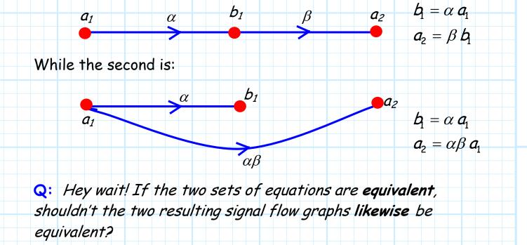
A: Absolutely! The two signal flow graphs are indeed equivalent.
