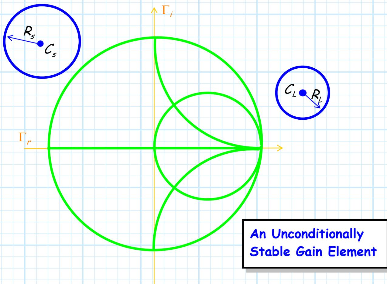
For this condition, we find that the values of  $\Gamma_L$  and  $\Gamma_s$  that result in an unstable amplifier must have a magnitude **greater than 1** (i.e.,  $|\Gamma_L| > 1$  or  $|\Gamma_s| > 1$ ).
