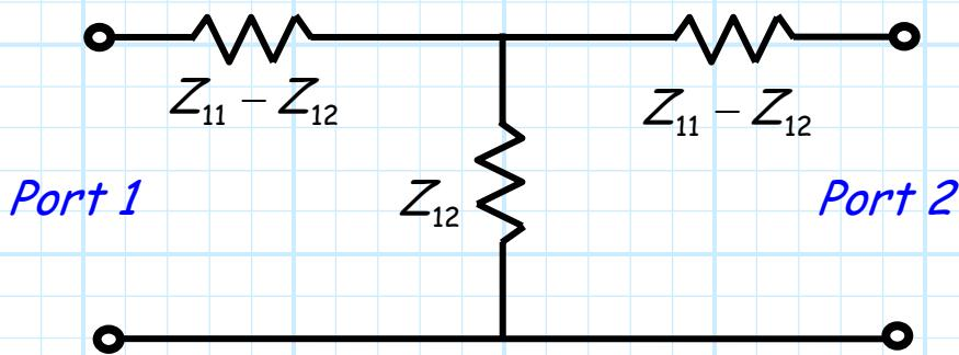
In other words, if the two **series impedances** have an impedance value equal to  $Z_{11} - Z_{21}$ , and the **shunt impedance** has a value equal to  $Z_{21}$ , the impedance matrix of this "T-circuit" is:
