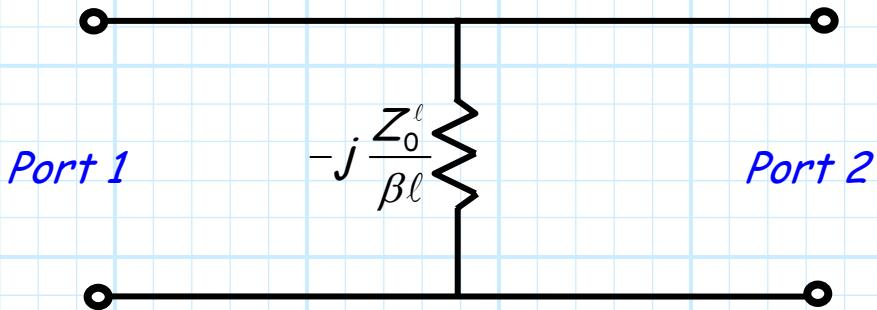
The equivalent circuit for transmission line with short electrical length ( $\beta\ell \ll 1$ ) and small characteristic impedance  $Z_0^\ell$  ( $Z_0^\ell \ll Z_0$ ).
