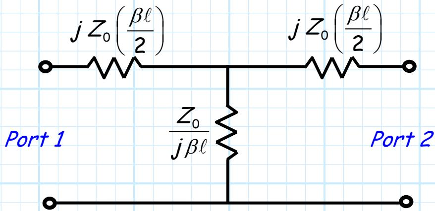
Now, consider also the case where the **characteristic impedance of the transmission line is relatively large**. We'll denote this large characteristic impedance as  $Z_0^h$ .
