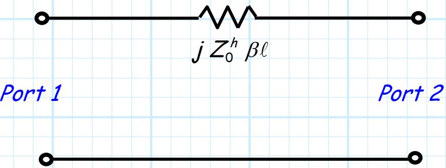
*The equivalent circuit for transmission line with short electrical length ( $\beta l \ll 1$ ) and large characteristic impedance  $Z_0^h$  ( $Z_0^h \gg Z_0$ ).*
