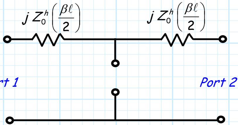
The remaining impedances are now in **series**, so the circuit can be further simplified to:
