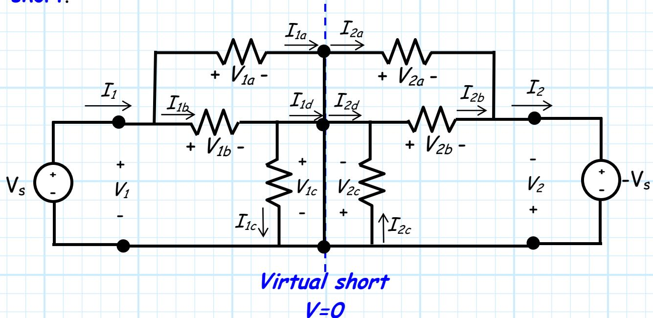
This **greatly simplifies** things, as we can again **break** the circuit into **two** independent and (effectively) identical circuits!
