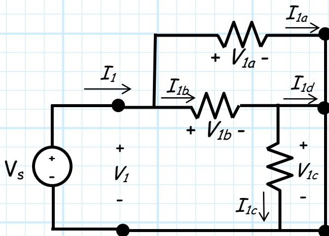
$$\begin{aligned} I_1 &= V_s / 50 \\ I_{1a} &= V_s / 100 \\ I_{1b} &= V_s / 100 \\ I_{1c} &= 0 \\ I_{1d} &= V_s / 100 \end{aligned}$$
