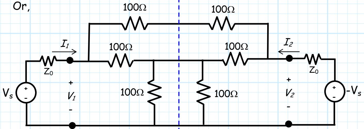
This situation still preserves the **symmetry** of the circuit—somewhat. The voltages and currents in the circuit will now possess **odd symmetry**—they will be **equal but opposite** (180 degrees out of phase) at symmetric points across the symmetry plane.
