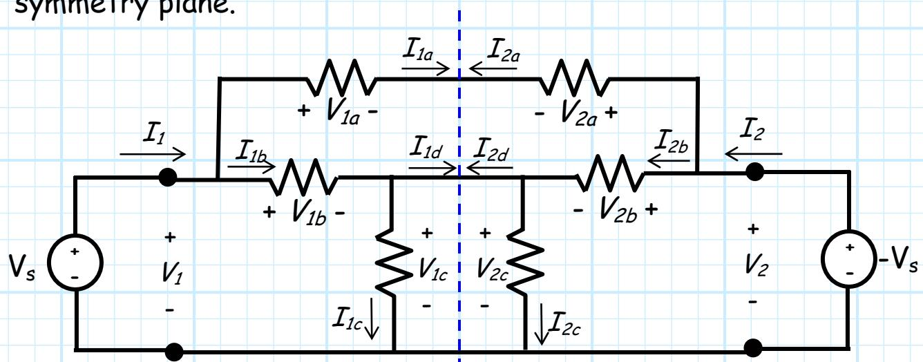
$$\begin{aligned} V_1 &= -V_2 \\ V_{1a} &= -V_{2a} \\ V_{1b} &= -V_{2b} \\ V_{1c} &= -V_{2c} \end{aligned}$$
