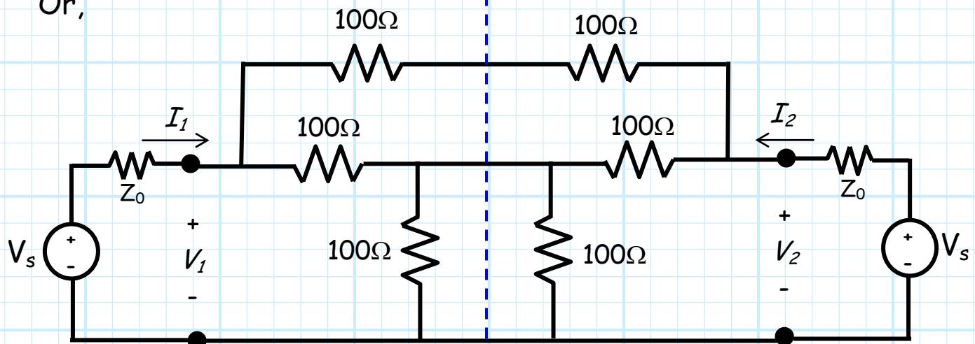
But remember! In order for **symmetry to be preserved**, the source values on both sides (i.e.,  $I_s, V_s, Z_0$ ) must be **identical**!
