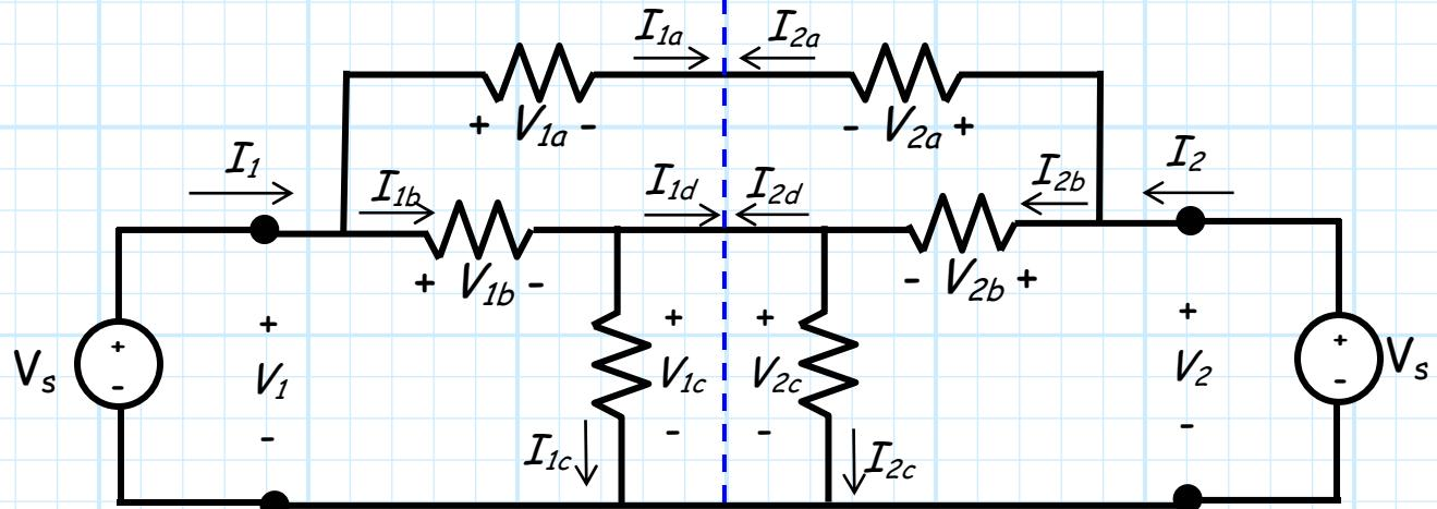
Since this circuit possesses **bilateral** (reflection) symmetry ( $1 \rightarrow 2, 2 \rightarrow 1$ ), symmetric currents and voltages must be equal:
