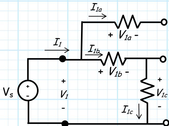
$$V_1 = V_2 = V_s$$
