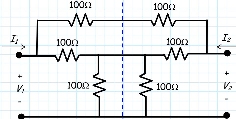
Recall that the **symmetry** of this 2-port device leads to simplified network matrices:
