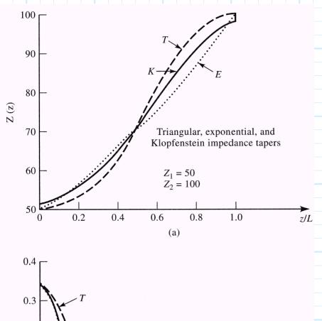
$0.3 \qquad T$   $0.1 \qquad K$   $0.1 \qquad \pi \qquad 2\pi \qquad 3\pi \qquad 4\pi \qquad 5\pi \qquad 6\pi \qquad \beta L$ Passband of K taper
