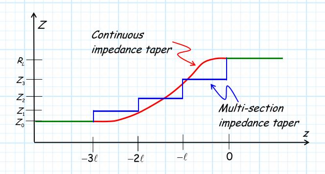
A tapered impedance matching network is defined by **two** characteristics—its **length** L and its taper **function**  $Z_1(z)$ :
