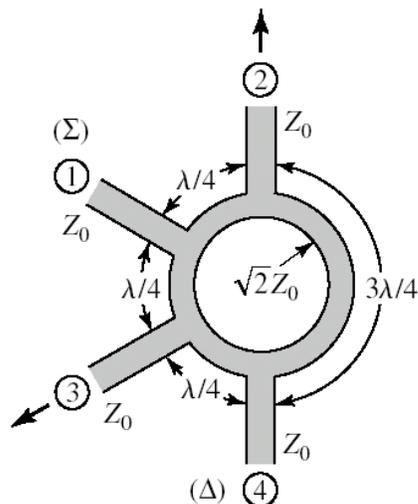
**A:** Like the quadrature hybrid, it is simply made of **lengths** of transmission lines. However, unlike the quadrature hybrid, the characteristic impedance of each line is **identical** ( $\sqrt{2}Z_0$ ), but the lengths of the lines are dissimilar.
