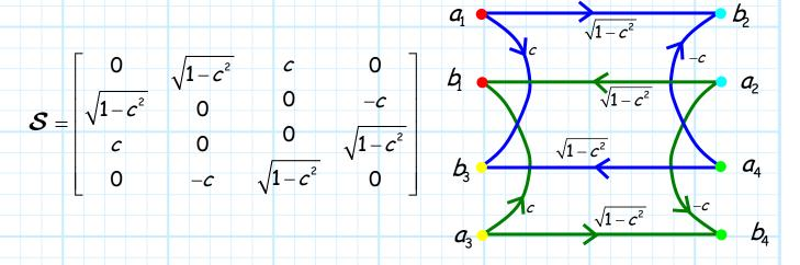
Additionally, for a directional coupler, the coupling coefficient c will be less than  $1/\sqrt{2}$  always. Therefore, we find that:
