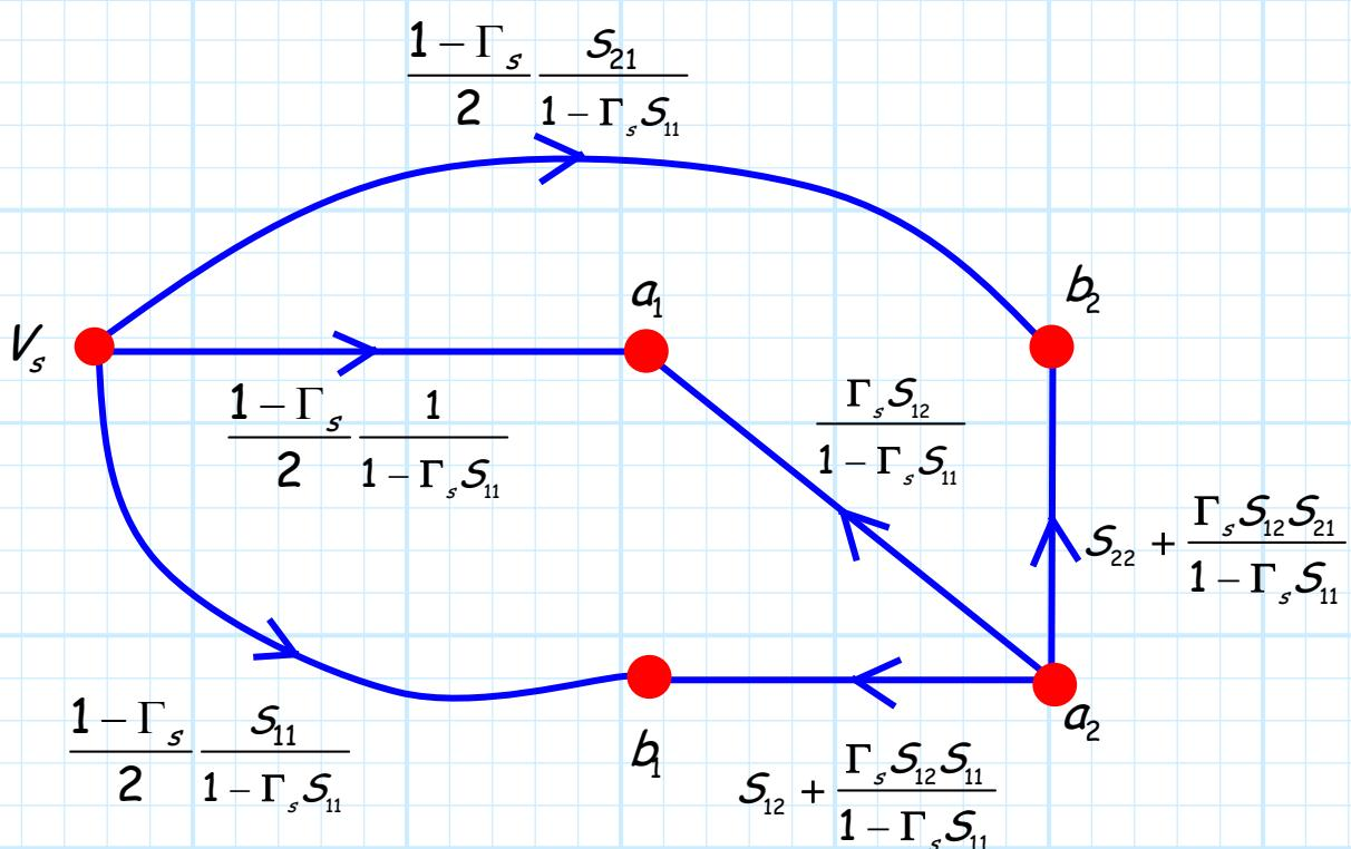
Now, for the purposes of determining the output power at port 2, we can ignore nodes  $a_1$  and  $b_1$  (in the final signal flow-graph above they are terminal nodes, no branches are leaving these nodes). Thus, the relevant portion of the reduced signal flow graph is:
