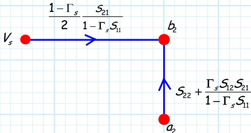
Notice this signal flow graph has the same form as the source signal-flow graph:
