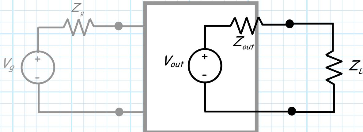
These four power quantities depend (at least in part) on the source parameters  $V_g$  and  $Z_g$ , load  $Z_L$ , and the scattering parameters of  $S_{11}, S_{21}, S_{22}, S_{12}$  the gain element.
