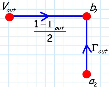
It is apparent that  $V_{out}$  and  $\Gamma_{out}$  define an **equivalent source** created when the original source is connected to a two-port device.
