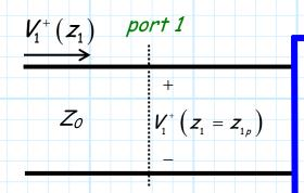
Say we measure/determine the voltage of the wave flowing into port 1, at the port 1 plane (i.e., determine  $V_1^+(z_1=z_{1\rho})$ ).
