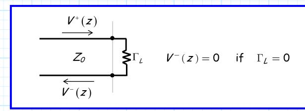
In this original case, the wave incident on the load is  $V^+(z)$  (plus direction), while the reflected wave is  $V^-(z)$  (minus direction).
