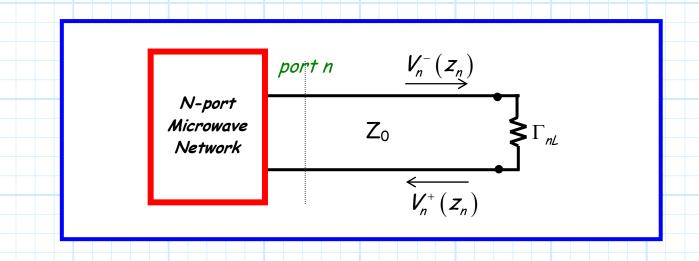
For this current case, the situation is **reversed**. The wave incident on the load is **now** denoted as  $V_n^-(z_n)$  (coming **out** of port n), while the wave reflected off the load is **now** denoted as  $V_n^+(z_n)$  (going **into** port n).
