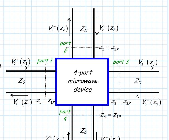
Say there exists an **incident** wave on **port 1** (i.e.,  $V_1^+(z_1) \neq 0$ ), while the incident waves on all other ports are known to be **zero** (i.e.,  $V_2^+(z_2) = V_3^+(z_3) = V_4^+(z_4) = 0$ ).
