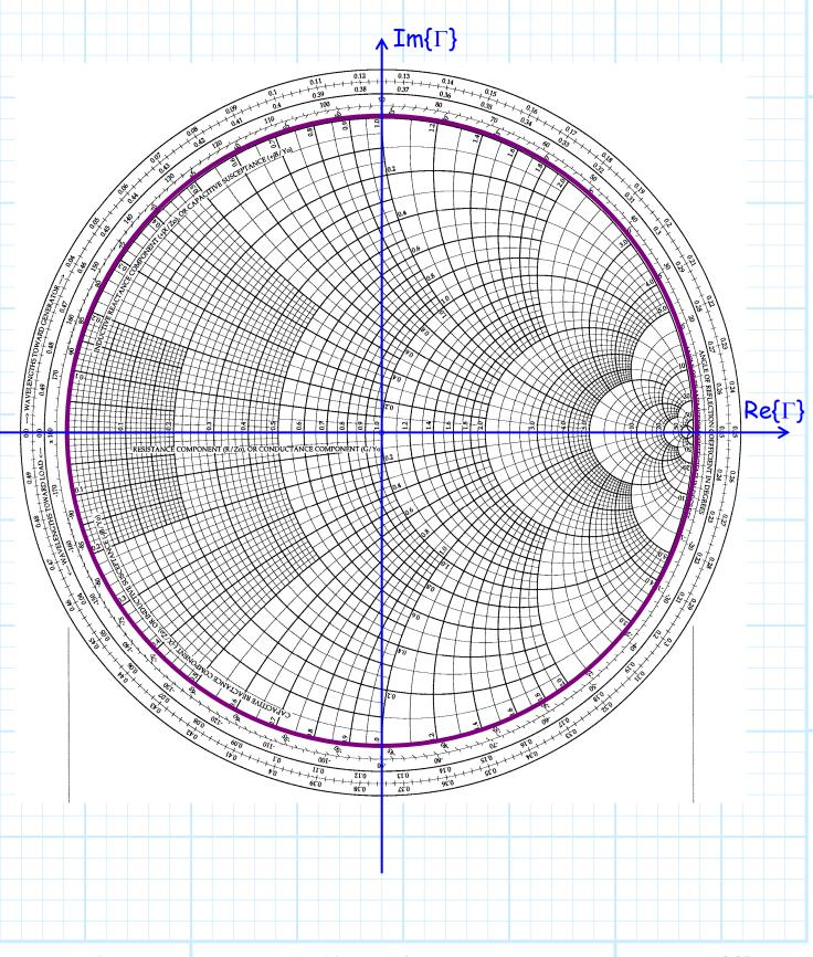
Note the Smith Chart is simply the vertical lines  $r = c_r$  and horizontal lines  $x = c_i$  of the normalized **impedance** plane, **mapped** onto the two types of **circles** on the complex  $\Gamma$  plane.
