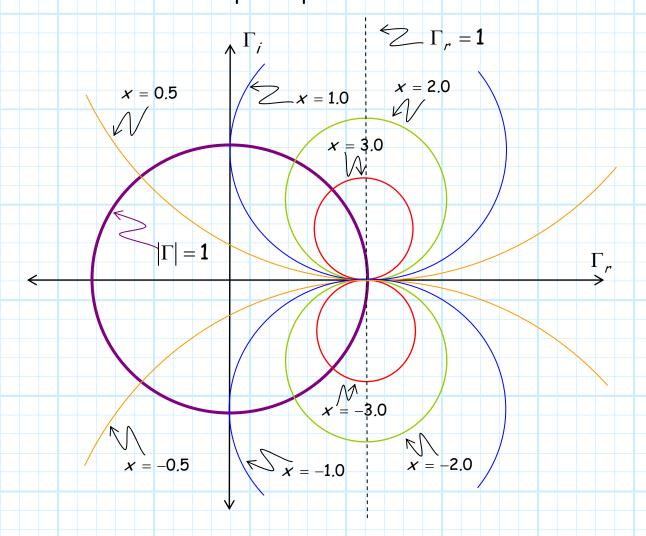
We see that as the **magnitude** of constant  $c_i$  increases, the radius of the circle **decreases**, and its **center** moves toward the point  $(\Gamma_r = 1, \Gamma_i = 0)$ .
