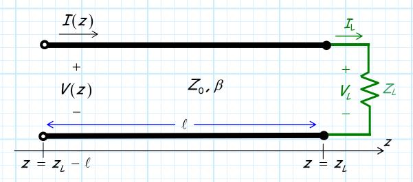
Q: What is the **current** and **voltage** at each and **every** point on the transmission line (i.e., what is I(z) and V(z) for **all** points z where  $z_L - \ell \le z \le z_L$ ?)?
