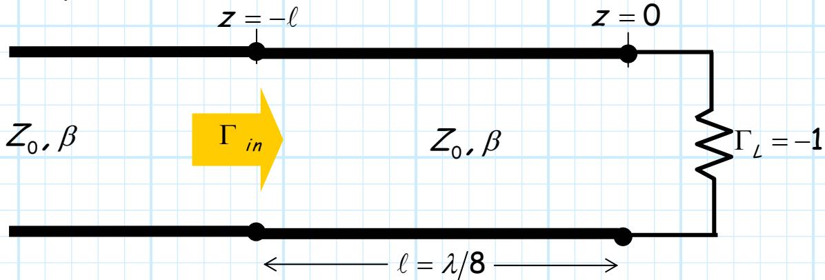
The reflection coefficient of a short circuit is  $\Gamma_L = -1 = 1 e^{j\pi}$ , and therefore we begin at that point on the complex  $\Gamma$  plane. We then move along a circular arc  $-2\beta\ell = -2(\pi/4) = -\pi/2$  radians (i.e., rotate clockwise  $90^\circ$ ).
