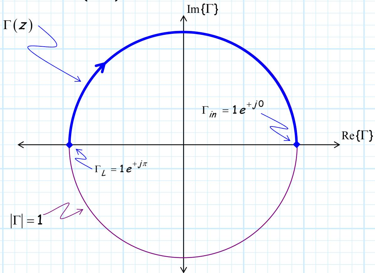
For this case, the **input** reflection coefficient is  $\Gamma_{in} = 1 e^{j0} = 1$  : the reflection coefficient of an **open circuit**!
