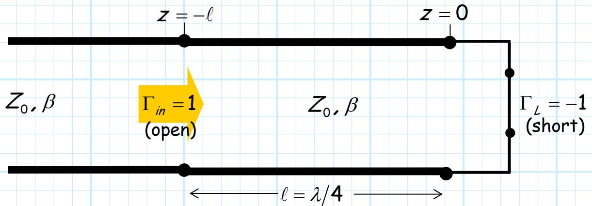
Recall that a **quarter-wave** transmission line was one of the **special cases** we considered earlier. Recall we found that the input impedance was proportional to the **inverse** of the load impedance.
