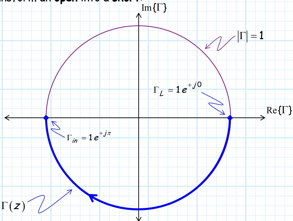
Finally, let's again consider the problem where  $\Gamma_L = -1$  (i.e., short), only this time with a transmission line length  $\ell = \lambda/2$  (a half wavelength!). We rotate clockwise  $2\beta\ell = 2\pi$  radians ( $360^\circ$ ).
