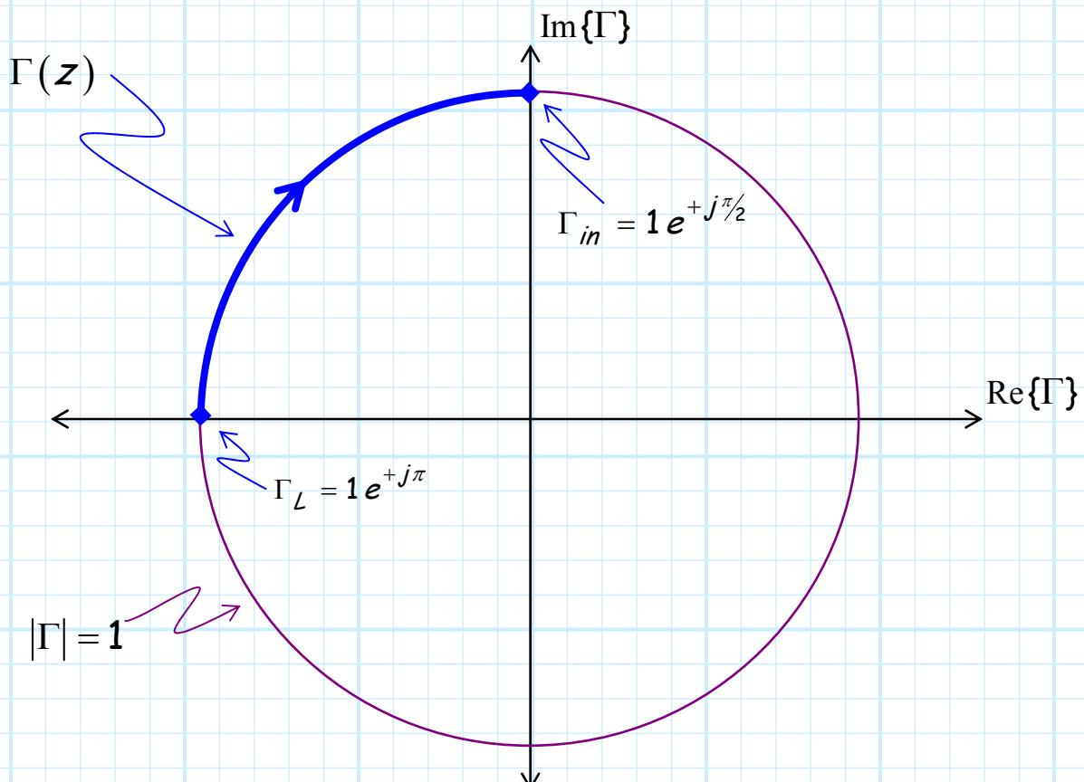
When we **stop**, we find we are at the point for  $\Gamma_{in}$ ; in this case  $\Gamma_{in} = 1 e^{j\pi/2}$  (i.e., magnitude is **one**, phase is **90°**).
