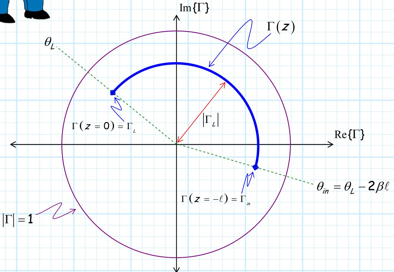
Since adding a length of transmission line to a load  $\Gamma_L$  modifies the phase  $\theta_\Gamma$  but not the magnitude  $|\Gamma_L|$ , we trace a circular arc as we parametrically plot  $\Gamma(z)$ ! This arc has a radius  $|\Gamma_L|$  and an arc angle  $2\beta\ell$  radians.
