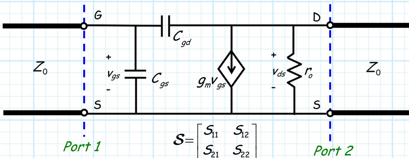
We can determine this scattering matrix either by direct **measurement** (using a network analyzer) or by **analysis** of the small-signal circuit.
