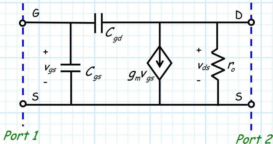
where again  $g_m$ ,  $r_o$  are small-signal parameters and  $C_{gs}$ ,  $C_{gd}$  are parasitic elements.
