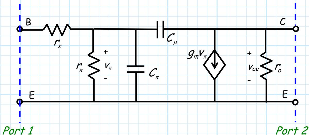
Here the values  $g_m, r_\pi, r_o$  are all **small-signal parameters**—values determined in part by the **DC bias** of the transistor.
