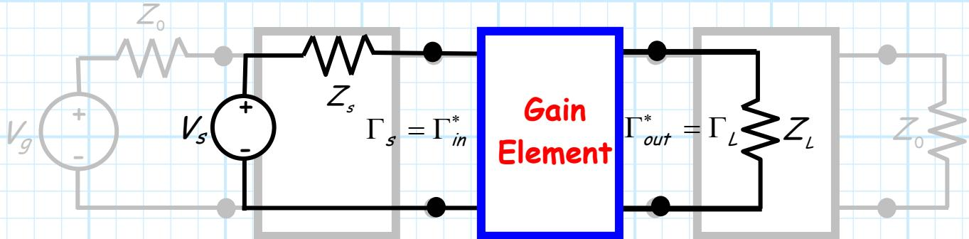
where the values of  $\Gamma_s$  and  $\Gamma_L$  depend on the input and output matching networks.
