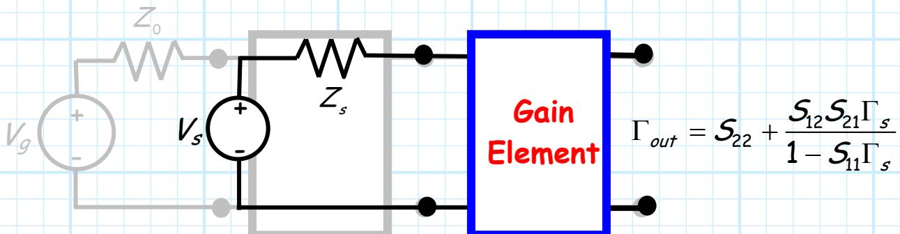
Likewise, the value of  $\Gamma_{in}$  depends on the value of  $Z_L$  (i.e., depends on  $\Gamma_L$ ).
