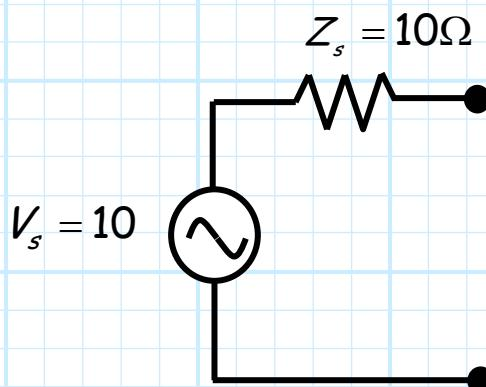
$$\begin{aligned} P_{avs} &= \frac{|V_s|^2}{8 \operatorname{Re}\{Z_s\}} \\ &= \frac{10^2}{8(10)} \\ &= 1.25 \text{ W} \end{aligned}$$
