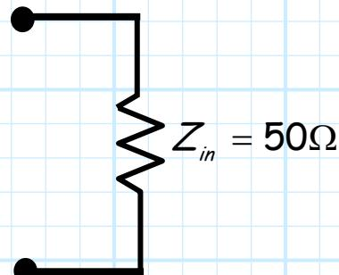
Although increasing the source impedance by  $40 \Omega$  would result in a **conjugate match**, it would likewise **reduce** the available power to a measly **0.25 Watts**.
