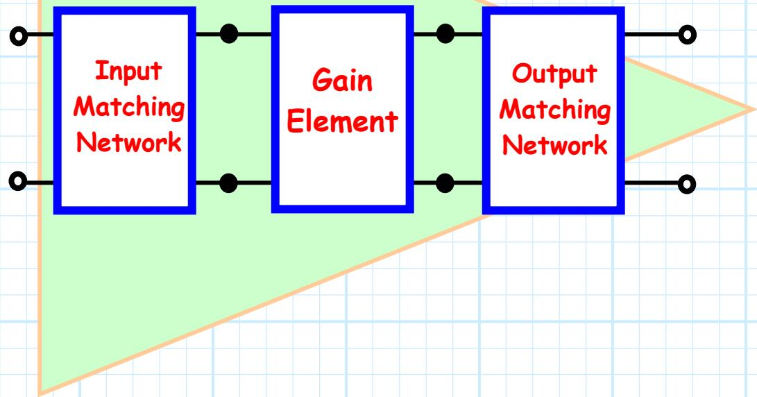
Of course, the impedance of both the source and the load connected to this amp will most certainly be that of transmission line **characteristic impedance**  $Z_0$ . Thus, our amplifier circuit is typically:
