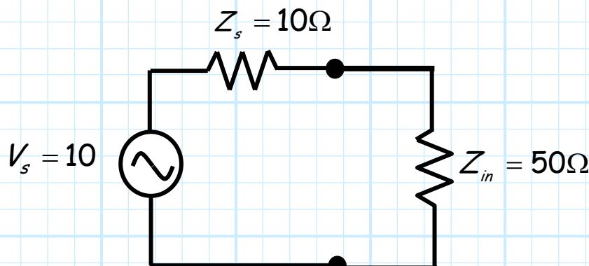
$$\begin{aligned} P_L &= \frac{1}{2} |V_g|^2 \frac{\operatorname{Re}\{Z_L\}}{|Z_g + Z_L|^2} \\ &= \frac{10^2}{2} \frac{50}{(20 + 50)^2} \\ &= \frac{50^2}{70^2} \\ &= 0.51 \text{ W} \end{aligned}$$
