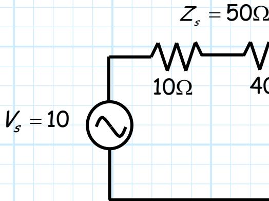
$$\begin{aligned} P_{av} &= \frac{|V_s|^2}{8 \operatorname{Re}\{Z_s\}} \\ &= \frac{10^2}{8(50)} \\ &= 0.25 \text{ W} \end{aligned}$$
