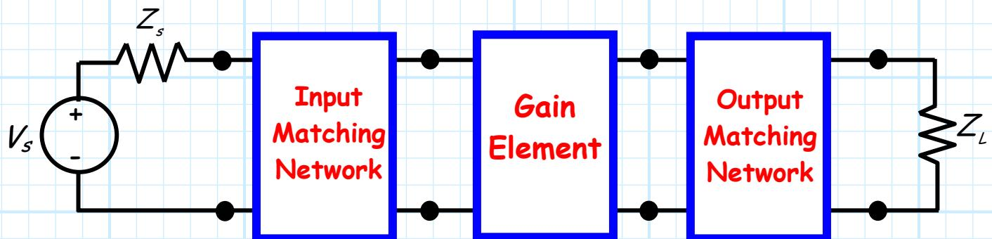
The **three stages** together—input matching network, gain element, and output matching network—form a **microwave amplifier**!
