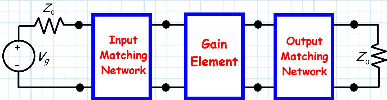
The **input network** is thus required to match  $Z_0$  to the gain element input impedance  $Z_{in}$ . For the purposes of amplifier design, we view the input matching network as one that transforms the source impedance  $Z_0$  into a new source impedance  $Z_s$ , one that is conjugate matched to the gain element input impedance  $Z_{in}$ :
