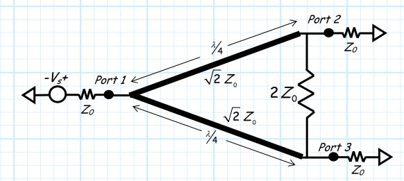
Note this source does **not** alter the bilateral symmetry of the circuit. We can thus use this symmetry to **help analyze** the circuit, **without** having to specifically define odd and even mode sources.
