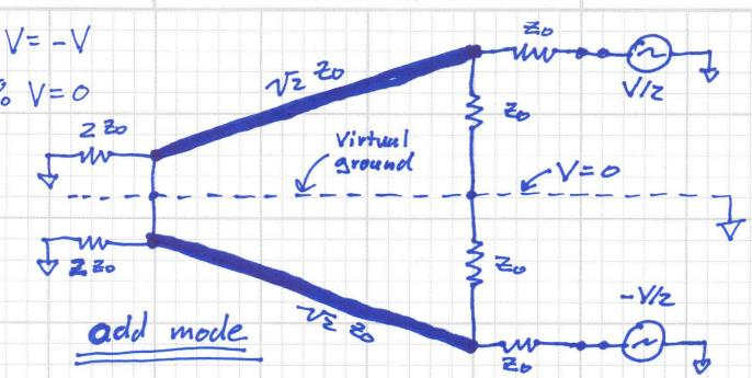
We call this odd mode symmetry plane a virtual short, as the voltage along this plane must be zero. As a result, we can divide the odd mode circuit into two pieces:
