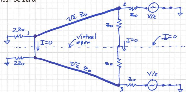
We call this even mode symmetry plane a virtual open, as the current along this plane must be zero. As a result, we can divide the even mode circuit into two pieces:
