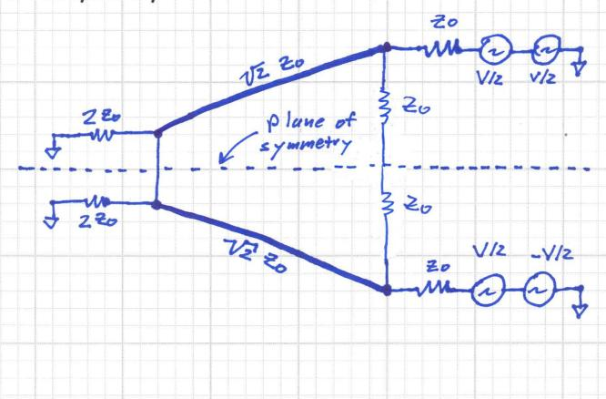
Consider now this symmetry with respect to the **odd** mode. It is evident that at **every** point along this symmetry plane, the **voltage** must be **zero**!
