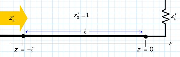
The normalized input impedance  $z_{in}'$  of a transmission line length  $\ell$ , when terminated in normalized load  $z_{\ell}'$ , can be determined as:
