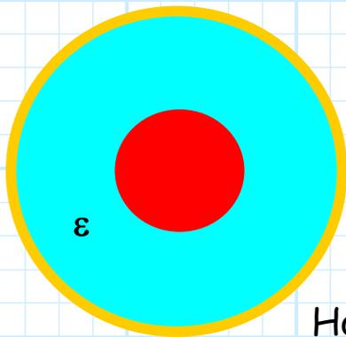
For example, a **coaxial** line has an inner conductor (**conductor #1**) and an outer conductor (**conductor #2**), with the cylindrical space between filled with dielectric.
