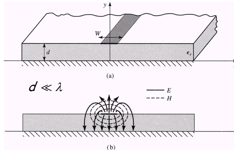
There are no **exact** analytic solutions for a microstrip transmission line—they must be **numerically** analyzed. However, we can use those results to form an analytic **approximation** of microstrip transmission line behavior.
