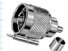
The **original** microwave connector. Good performance (up to 18GHz), and moderate cost, but large (about 2 cm in diameter)! However, can handle greater **power** than SMA.
