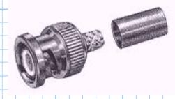
BNC The workhorse RF connector. Relatively small and cheap, and easy to connect. Don't use this connector past 2 GHz!
