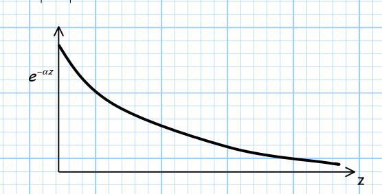
Therefore,  $\alpha$  expresses the **attenuation** of the signal due to the loss in the transmission line.
