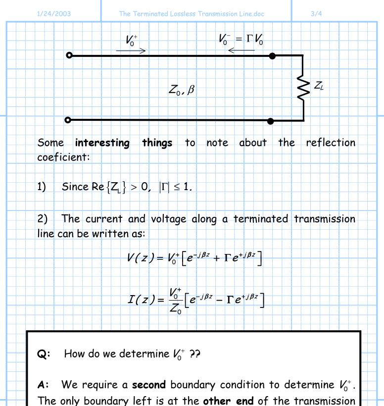
The only boundary left is at the **other end** of the transmission line. Typically, a **source** of some sort is located there. This makes physical sense, as something must generate the **incident** wave !
