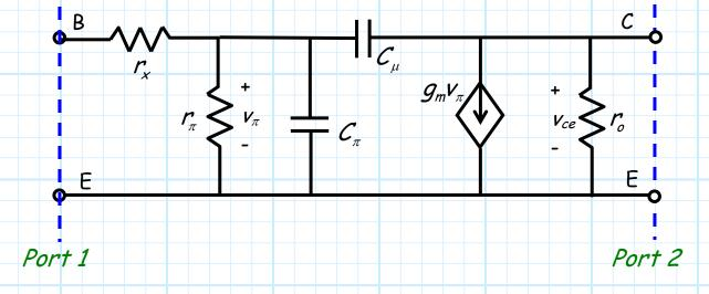
Here the values  $g_m, r_\pi, r_o$  are all small-signal parameters values determined in part by the DC bias of the transistor.
