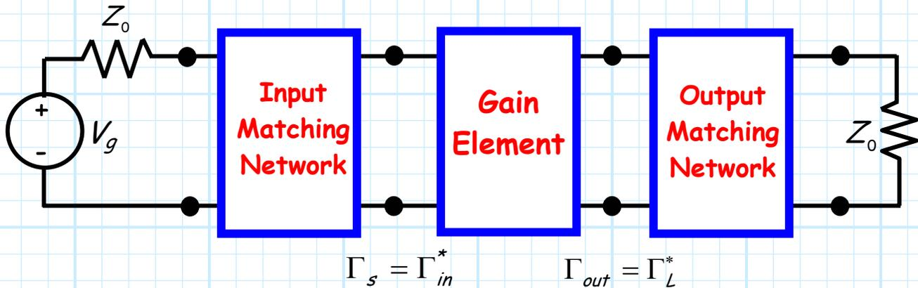
**Q:** So if we design our amplifier such that the source is **matched** to the input of the gain element, and the output of the gain element is **matched** to the load, what is the resulting gain?
