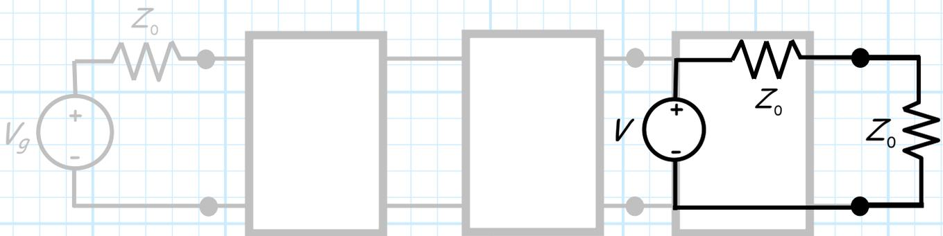
As a result, the scattering parameter  $S_{22}$  of the matched amplifier is also **zero!**
