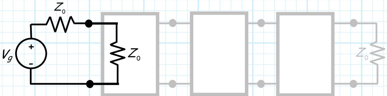
Meaning that the scattering parameter  $S_{11}$  of the matched amplifier is **zero!**
