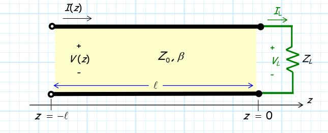
**Q:** What is the **current** and **voltage** at each and **every** point on the transmission line (i.e., what is I(z) and V(z) for **all** points z where  $-\ell \le z \le 0$  ?)?
