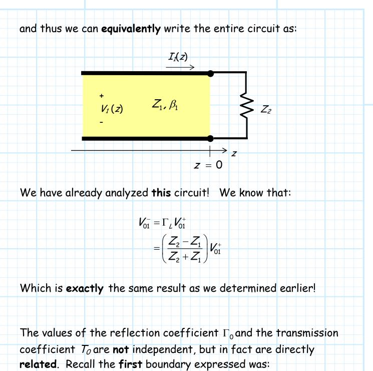
$$V_{01}^{+} + V_{01}^{-} = V_{02}^{+}$$
