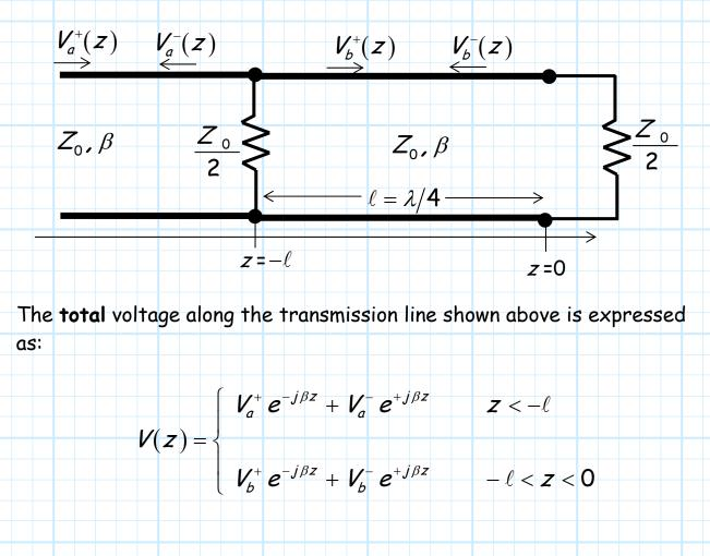
Carefully determine and apply boundary conditions at both z = 0 and  $z = -\ell$  to find the three values:
