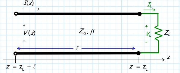
**Q:** What is the **current** and **voltage** at each and **every** point on the transmission line (i.e., what is I(z) and V(z) for **all** points z where  $z_{L} - \ell \le z \le z_{L}$ ?)?
