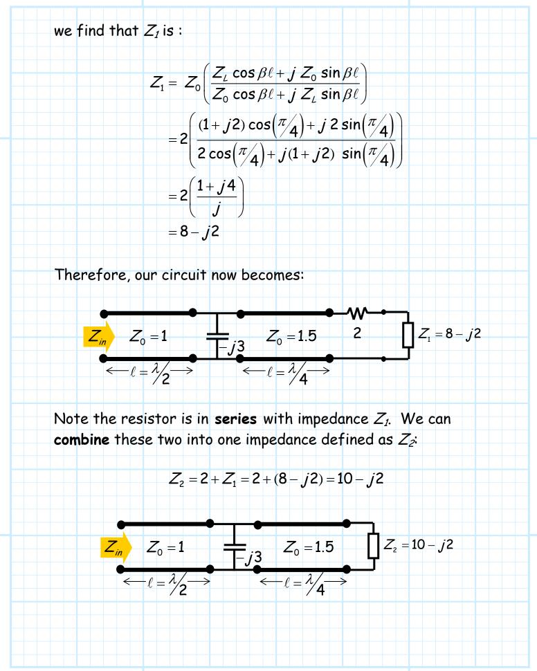
Now let's define the input impedance of the **middle** transmission line section as  $Z_3$ :
