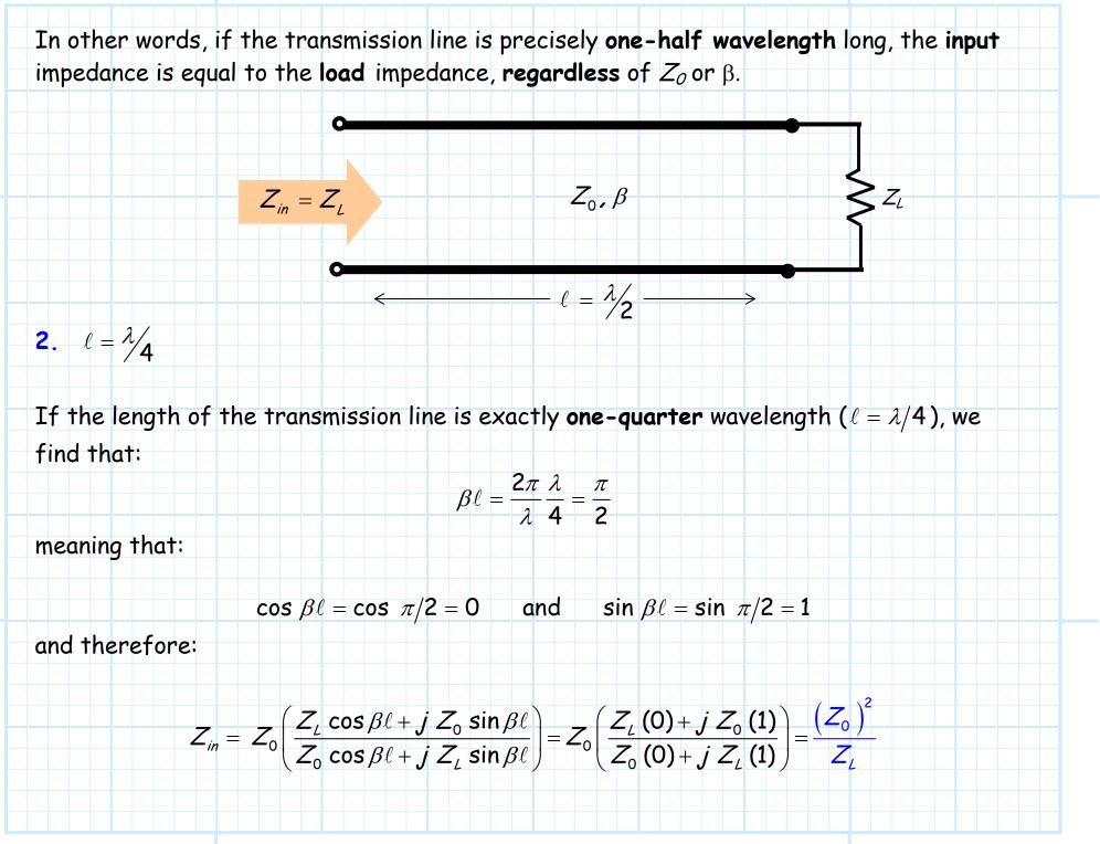
In other words, if the transmission line is precisely **one-quarter** wavelength long, the **input** impedance is **inversely** proportional to the **load** impedance.
