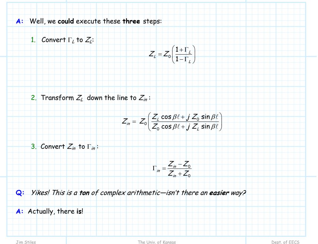
Recall in an **earlier handout** that the input impedance of a transmission line length l, terminated with a load  $\Gamma_L$ , is:
