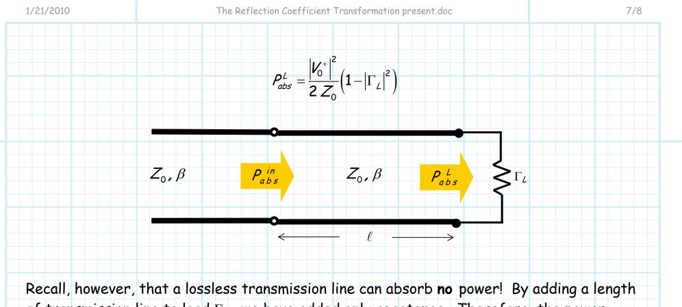
of transmission line to load  $\Gamma_L$ , we have added only **reactance**. Therefore, the power absorbed by load  $\Gamma_{in}$  is **equal** to the power absorbed by  $\Gamma_L$ :
