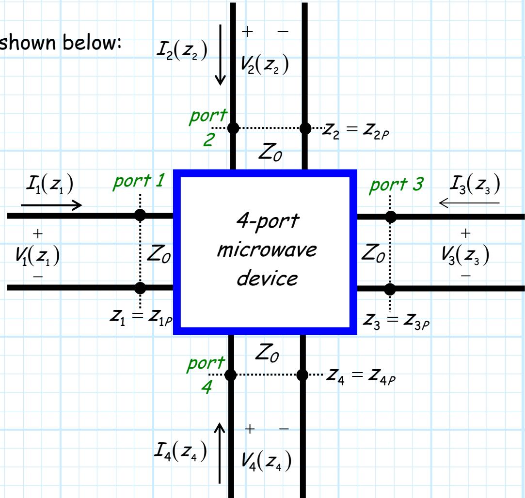
First, note that each transmission line has a specific **location** that effectively defines the **input** to the device (i.e.,  $z_{1P}$ ,  $z_{2P}$ ,  $z_{3P}$ ,  $z_{4P}$ ). These often arbitrary positions are known as the **port locations**, or **port planes** of the device.
