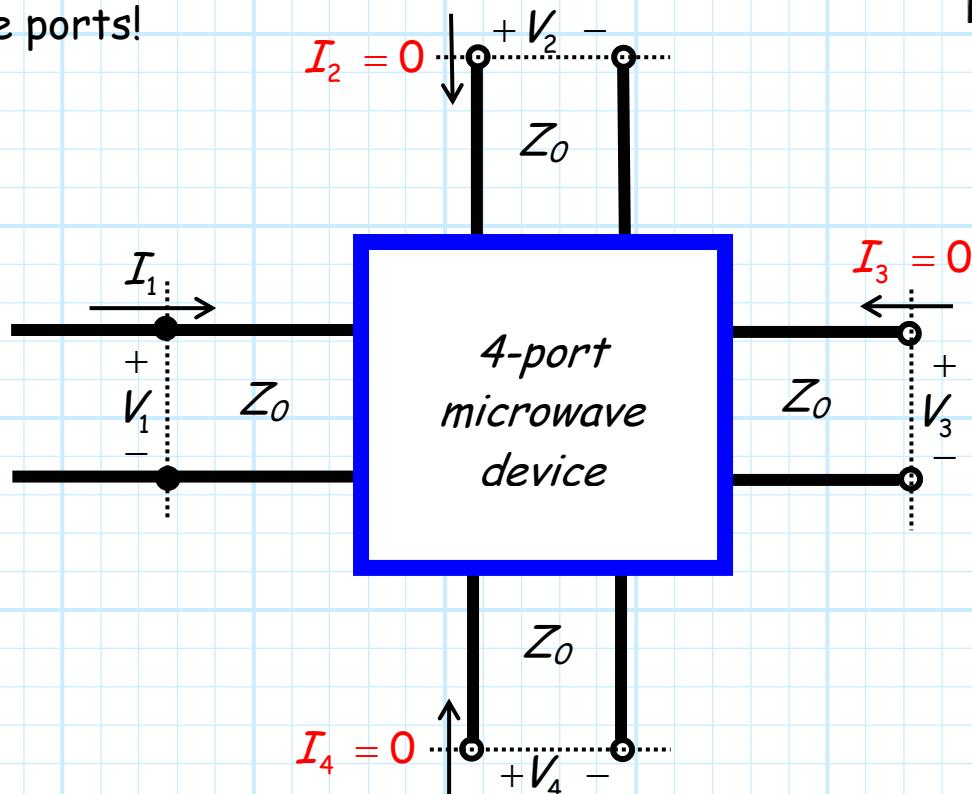
Placing an **open** at a port (and it must be **at the port!**) **enforces** the condition that  $I = 0$ .
