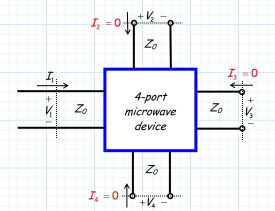
Placing an open at a port (and it must be at the port!) enforces the condition that I=0.
