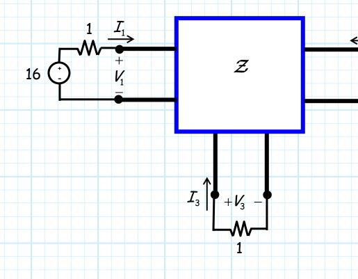
Where the 3-port device is characterized by the impedance matrix:
