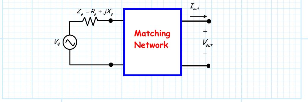
This "new" source (i.e., the original source with the matching network attached) can be expressed in terms of its Thevenin's equivalent circuit:  $Z_{out} = R_{out} + jX_{out}$  $V_{s}$ Note that in general that  $V_s \neq V_q$  and  $Z_{out} \neq Z_q$ —the matching network "transforms" both the values of both the impedance and the voltage source. **Q:** Arrrgg! Doesn't that mean that the available power of this "transformed" source will be different from the original?
