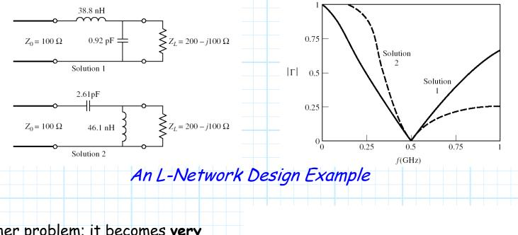
One other problem; it becomes very difficult to build quality lumped Lossy film elements with useful values past 1 or 2 GHz. Thus, L-Network solutions are Planar resistor generally applicable only in the RF region (i.e., < 2GHz). E Interdigital
