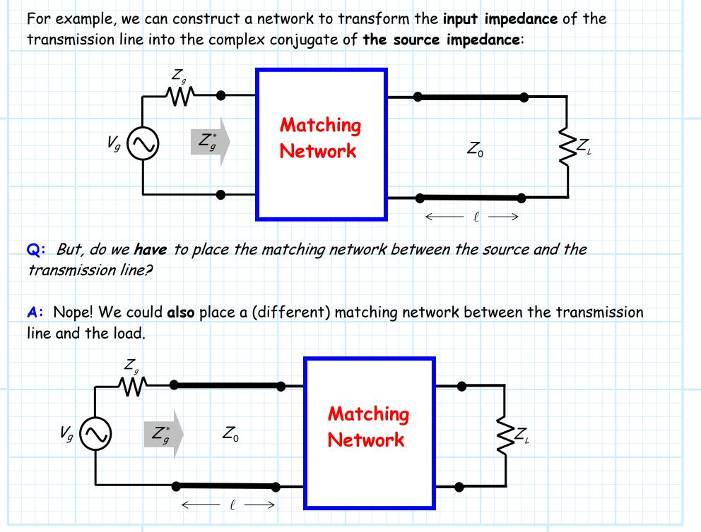
In either case, we find that at **any** and **all** points along this matched circuit, the output impedance of the equivalent **source** (i.e., looking left) will be equal to the **complex conjugate** of the **input** impedance (i.e., looking right).
