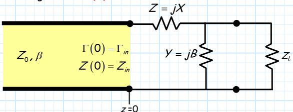
Note that this matching network consists of just two lumped elements, which must be purely reactive—in other words, a capacitor and an inductor!
