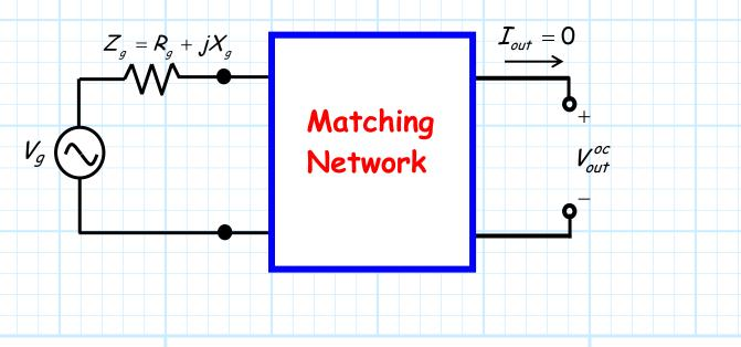
And likewise evaluating (or measuring) the **short-circuit** output **current**  $I_{out}^{sc}$ :
