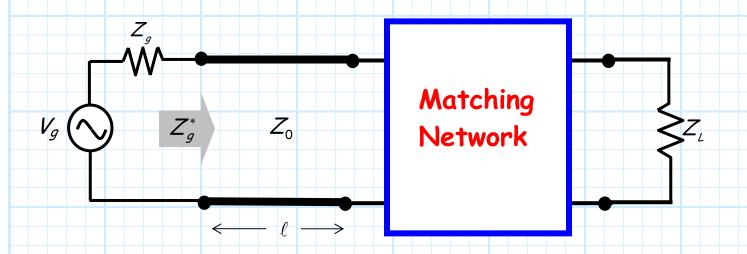
In either case, we find that at **any** and **all** points along this matched circuit, the output impedance of the equivalent **source** (i.e., looking left) will be equal to the **complex conjugate** of the **input** impedance (i.e., looking right).
