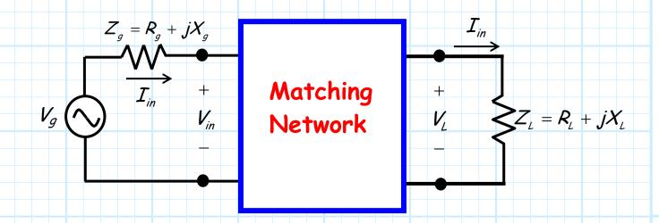
The sole purpose of this matching network is to "transform" the load impedance into an input impedance that is conjugate matched to the source! I.E.:
