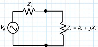
The load will absorb power—power that is delivered to it by the source.
