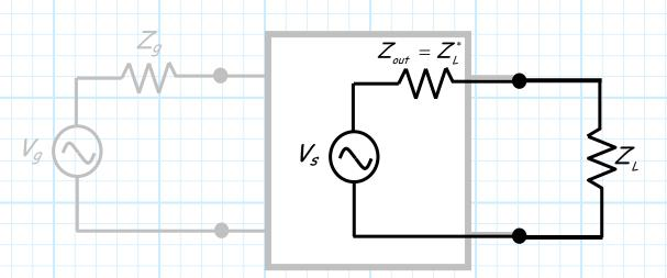
Either way, the source and load impedance are conjugate matched—all the available power is delivered to the load!
