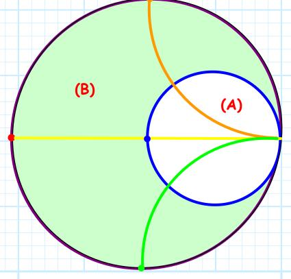
Once the values of X and B are found, we can determine the required values of inductance L and/or capacitance C, for the signal frequency  $\omega_0$ !
