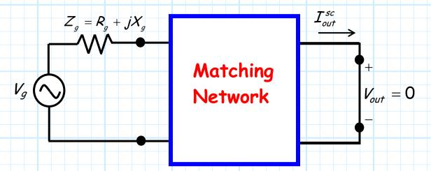
From these two values ( $V_{out}^{oc}$  and  $I_{out}^{sc}$ ) we can determine the **Thevenin's equivalent source**:
