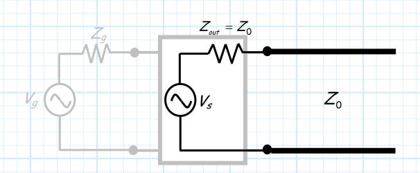
The second network matches the load to the transmission line—in other words it transforms the load impedance to a value numerically equal to characteristic impedance  $Z_0$ :
