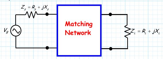
1. As a network attached to a load, one that "transforms" its impedance to  $Z_{in}$ —a value matched to the source impedance  $Z_{q}$ :
