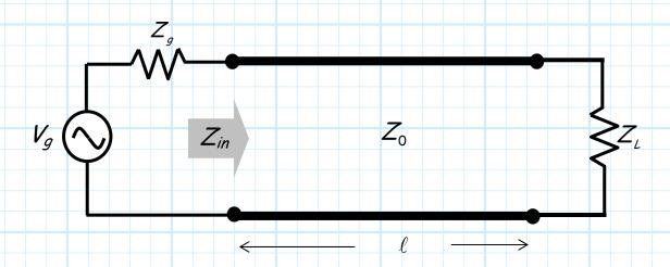
Q: So, say we directly connect an **arbitrary** source to an **arbitrary** load via a length of transmission line. Will the power delivered to the load be equal to the **available power** of the source?
