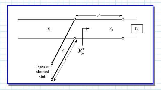
The two design parameters of this matching network are lengths  $\ell$  and d.
