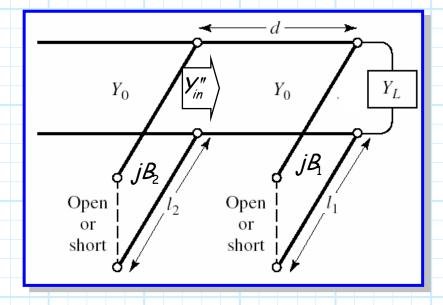
In this design, d is a **fixed** length (typically,  $d = \lambda/8$ ), whereas lengths  $\ell_1$  and  $\ell_2$  are **design parameters**.
