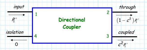
Note however, that **any** of the coupler ports can be an input, with a different through, coupled and isolation port for each case.
